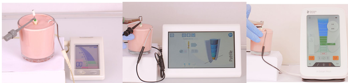
FIGURE 1 | Representative devices used for root canal length determination in a simulated root canal model. (Left) Standalone electronic apex locator (Root ZX Mini, J Morita Corp.) displaying real-time apex position feedback. (Centre) Endodontic motor with integrated apex locator (EnDrive, Komet Dental). (Right) Endodontic motor with integrated apex locator (X-Smart Pro+, Dentsply Sirona). All systems provide continuous electronic feedback during canal instrumentation.
